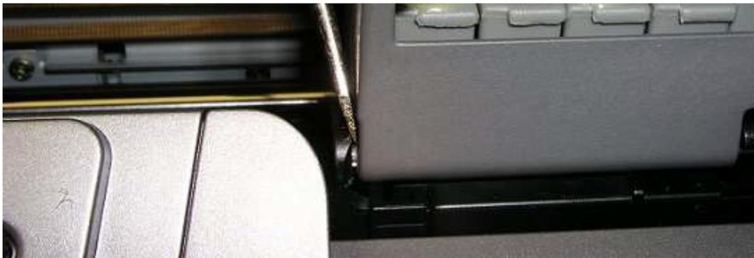
4. **PARTIALLY** install the CFS cartridges. Do not push the cartridges all the way down. We do not want the seals on the bottom to be punctured until the tubes have been installed in the bottles. In order to do this, you must follow these steps to route the tubing. The ends of the tubing with the blue clips should be on the left hand side of the printer.
