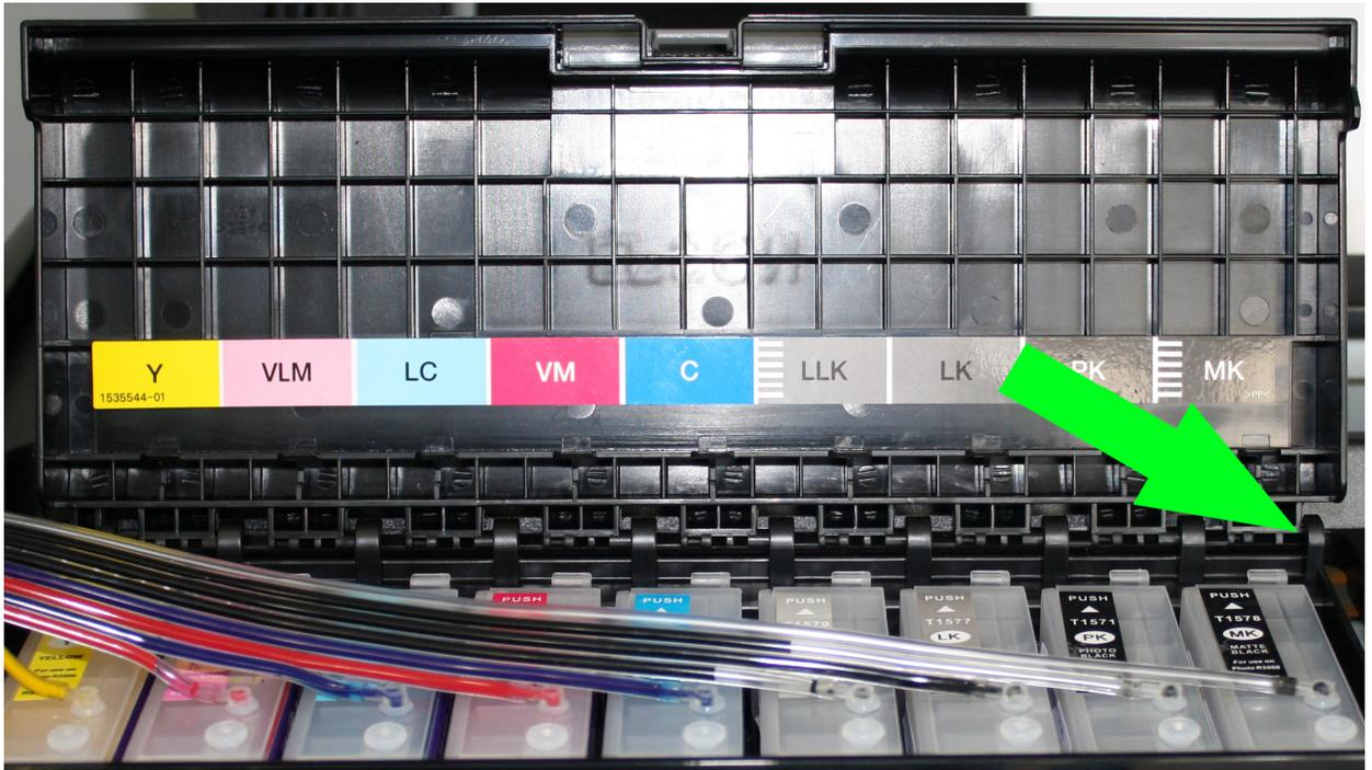
4. Next, carefully remove the ink carriage door by pulling the upper right corner free, and completely detaching the door.
