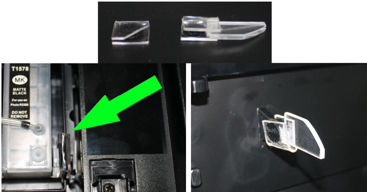
7. Install the cover switch activators. This is done by slipping the switch activator over the OEM activator, which is the protrusion on the underside of the printer lid. The second one is located on the right hand side of the cartridge carriage. This will allow the printer cover to sit flush as well as keep the cover switch activated to avoid printer errors.
