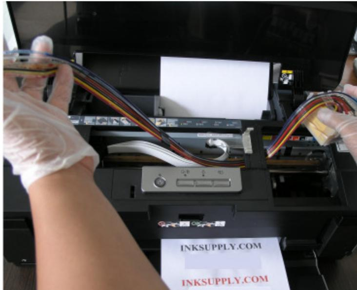
**Note:** This photo contains the R1900 CFS unit. Use photo for tube routing reference only.
