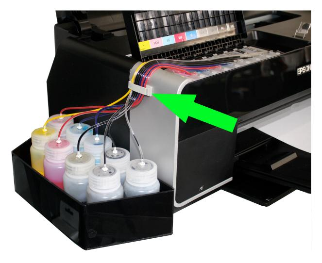
6. Peel the tubing on the bottle side of the ribbon back to the beige clip and begin installing the tubes to the bottles. Using scissors cut the tube to allow for a gentle curve down into the bottle.
