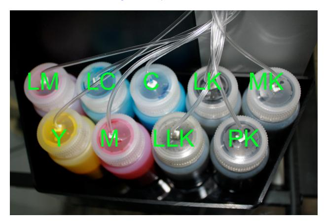
3. Arrange the bottles into the bottle holder in the orientation above. Color position is very important.
