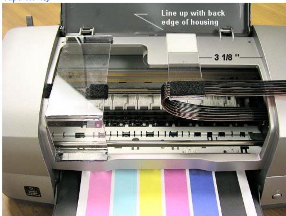
Use a pencil or marking pen, and mark a line on the printer housing, at 3 1/8 inches from the edge of the printer housing as shown in the above photo. This photo was taken after the tubes were installed.
