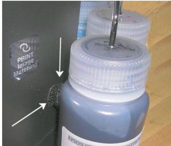
Velcro attaches bottles to printer
