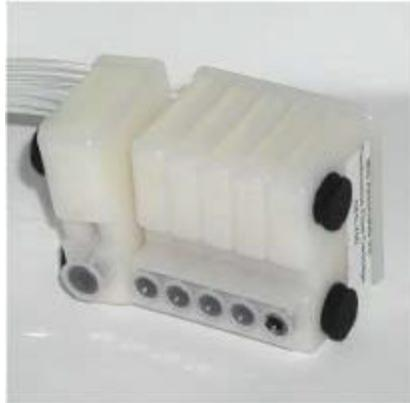
Detach the tube from the end of the Tube Adapter make sure it remains folded over and the vacuum is not lost. Insert the end of the tube at least one inch into the ink bottle without unfolding the bend (make sure it is the right color).
