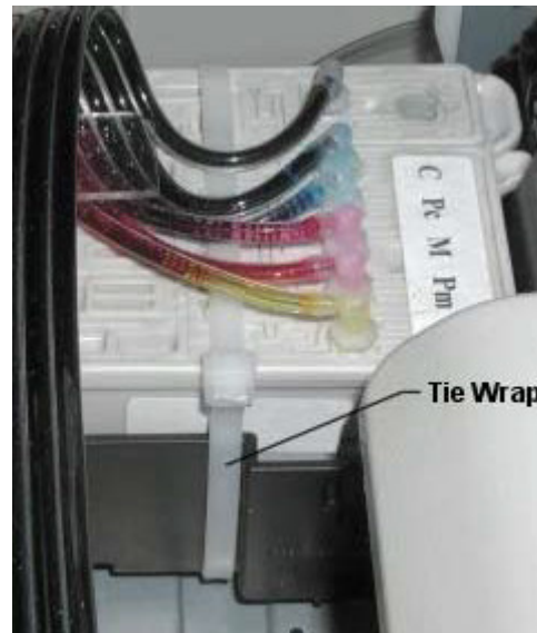
Tie Wrap Installation
