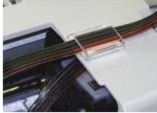
Use an alcohol swab to clean the plastic on the housing before attaching each bracket. Wipe the area dry with a paper towel after using alcohol swab. Once it goes down, it is there to stay, so don't put it in the wrong spot. This is important. If you have to remove it, use a wide blade screwdriver and twist it under the bracket. You can buy the white mounting tape at the hardware store if needed.
