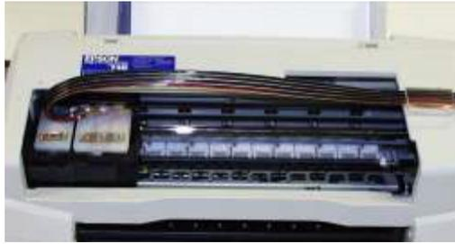
Clean off the excess lubricant or hand lotion from the tubing. You don't want the tubing to slip in the bracket as the cartridges move back and forth.
