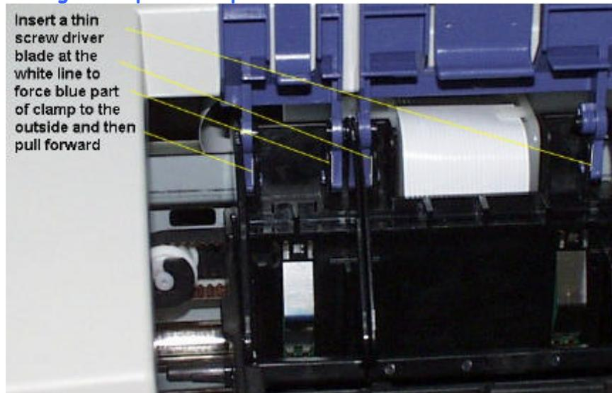
Push the paper feed button and hold it down for 3 seconds until the cartridge holder moves to the left. Pull the power plug out when the cartridge holder is in its remove position. This will keep it from returning to the right unexpectedly. **Don't plug the printer in again until later.**
