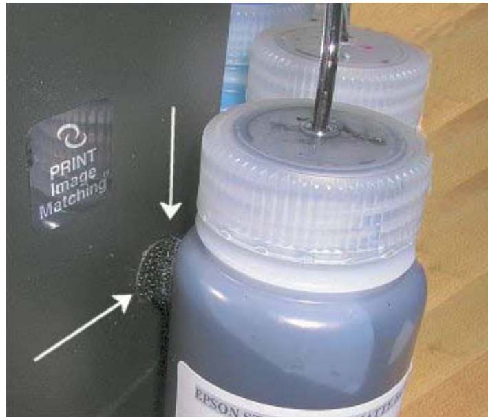
Velcro attaches bottles to printer
