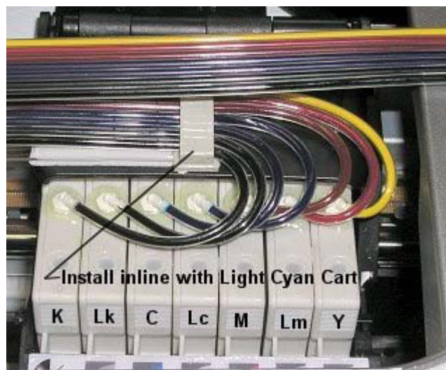
Photo taken after tubes installed
