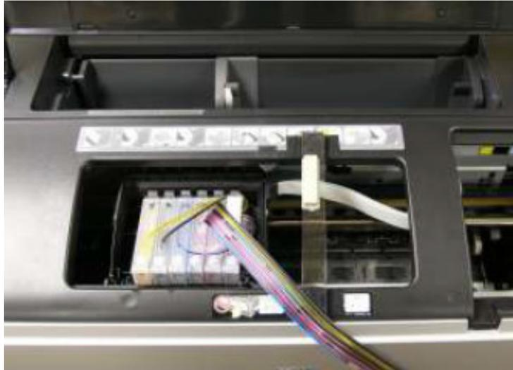
Install CFS cartridges
