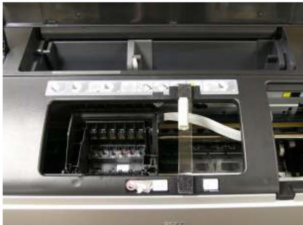
Move carriage with hand over to the left most access hole (center of printer)
