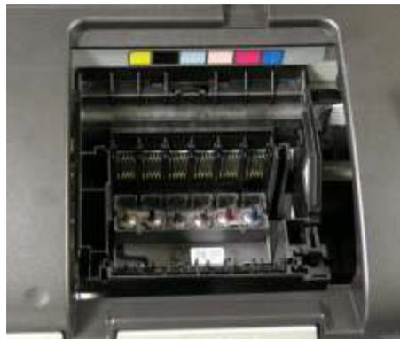
Remove OEM cartridges
