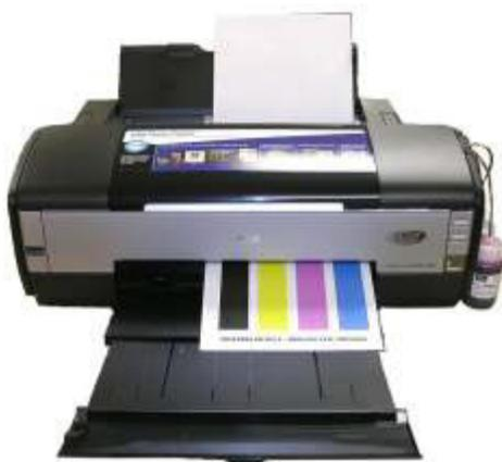
Epson 1400 with MIS CFS Installed
