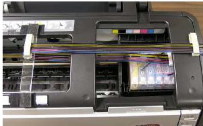
Proper tube installation
