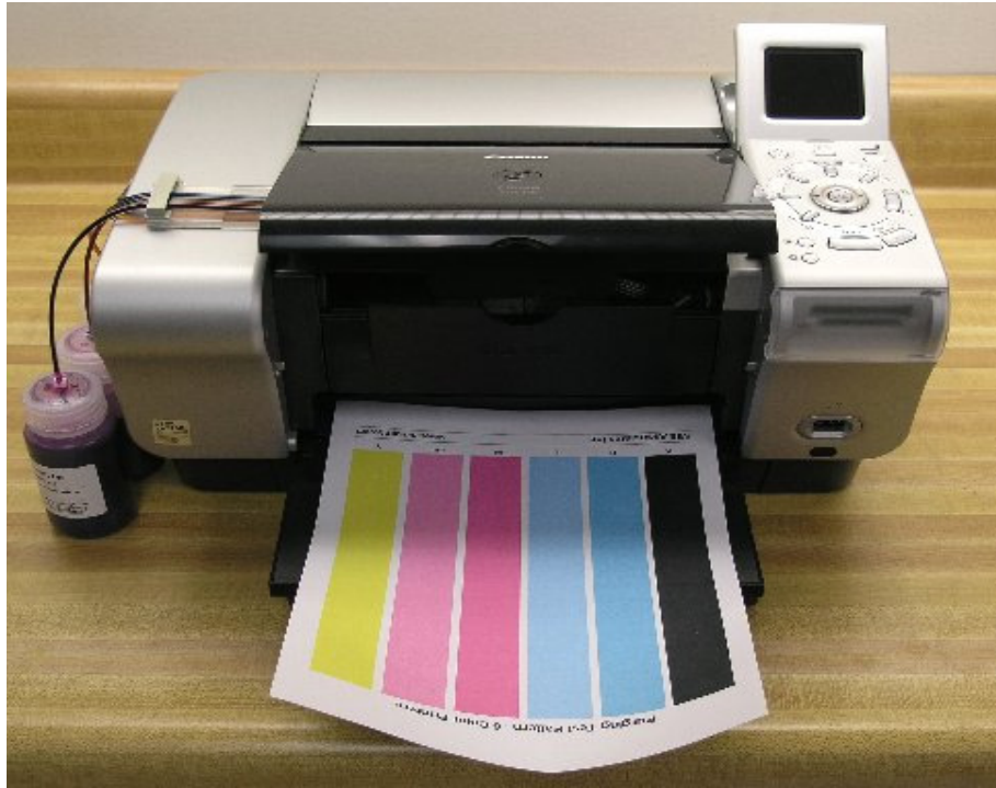
Canon Pixma iP6000 with MIS CFS Installed
