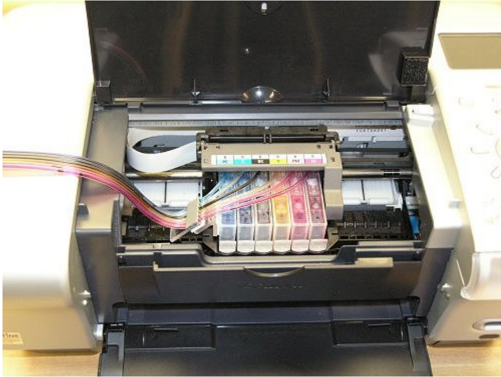
CFS Partially Installed
