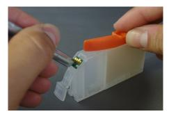
4. If the chip is loose, remove it and then use a SMALL amount of super glue or equivalent on the backside of the chip to keep it in place. **CAUTION:** Do not get any glue on the gold pads. If the chip snapped in place you will not need any glue.
