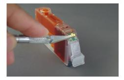
2. Use a knife blade or thin screwdriver blade to pry chip off of cartridge.
