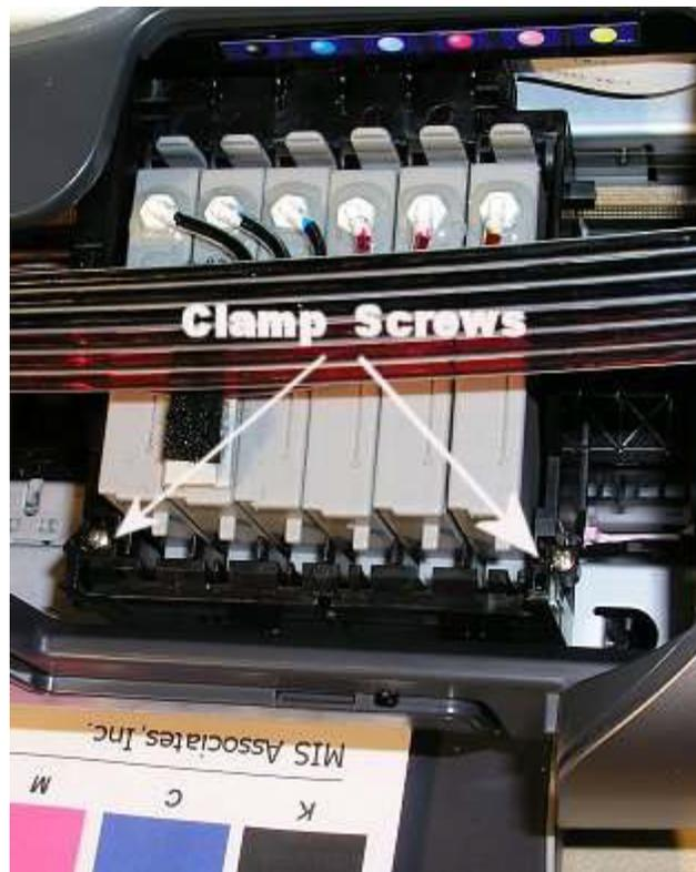
Clamp hinge screws on carriage
