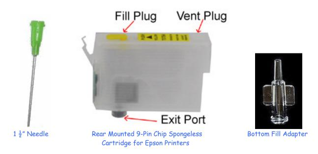
The Inksupply.com Empty Spongeless Cartridges for the Epson are a truly spongeless cartridge. These cartridges are designed to allow air to enter from the vent hole on the top of the cartridge and flow through a set of channels to the ink chamber at the very bottom of the cart. This prevents the print head from seeing any pressure thus eliminating siphoning issues.
