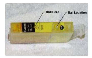
2. Use our black tool and a small hammer or equivalent device to push the ball into the reservoir. It does not take much, just one sharp blow right on the plastic ball. (See step 9 for alternative.)
