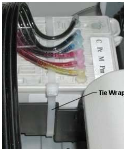
Tie Wrap Installation
