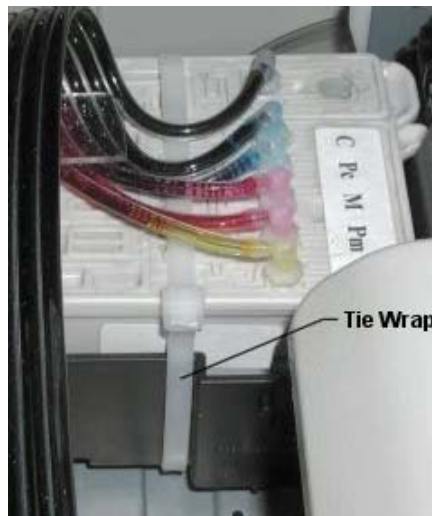
Tie Wrap Installation
