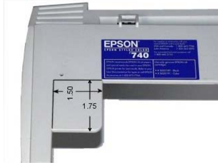
740 and 750 Require the Same Modification (740 shown here)
