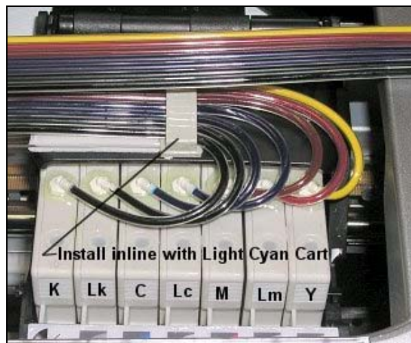
Photo taken after tubes installed
