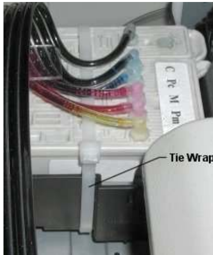
Tie Wrap Installation
